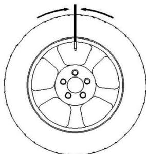
Turn the mouth of the wheel to the 12 point position, fix wheel then press [ok] for confirmation
