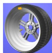
5. Manually rotate the wheel, when the outside counterweight position indicator lights turns to green, clip the counterweight in 12 o'clock direction.
