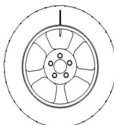
Rotate the wheel by hand, turn the balance block's position indicating piece to the top, and it turn to be red, keep the wheel's position, mark at the tire's 12 o'clock position, then take down the wheel, set it on the tire separating machine, and make the face to the air mouth of the rim.
