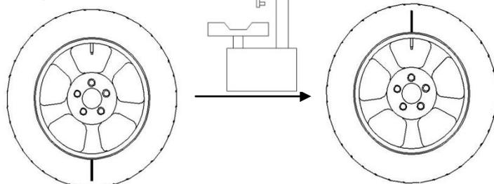
Take down the wheel, set it on the tire separating unit, and turn the related position between the tire and rim 180 degree.
