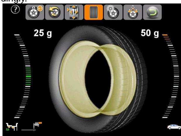
4. Tear the cover of the counterweight, clip the inside sticking weights with glue side up on the measuring ruler head. Rotate the wheel, when the inside counterweight position indicator lights on, pull out the measuring scale. When the inside counterweight position indicator lights turn to green, then stick the counterweight. There will be a bee sound when the user found the right position. After pasting, pull back the measuring scale, it will return to balancing page automatically.
