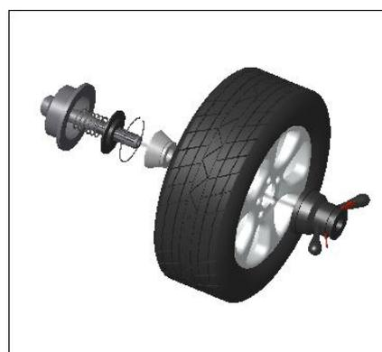
Main shaft -- spring (it has already been installed when the unite is manufactured),
