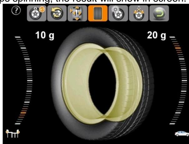
4. Manually rotate the wheel, when the inside counterweight position to green, clip the counterweight in 12 o'clock direction.
