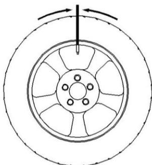
Turn the mouth of the wheel to 12 o'clock position, keep the wheel's position and confirm it by pressing OK. And the screen will show the rim's static unbalance mass, the tire's static unbalance mass, the current wheel's static unbalance mass, and the mix static unbalance mass that the wheel can reach. The user can decide to continue enhancing the wheel or not.
