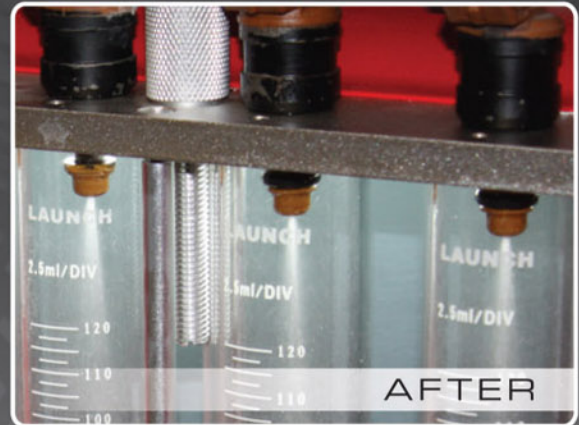
Back-lit: Graduated Cylinders Help To Accurately Diagnose Injector Flow Rates
