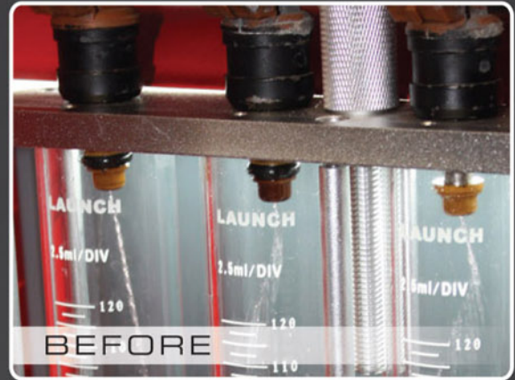
Back-lit: Graduated Cylinders Help To Accurately Diagnose Injector Flow Rates
